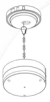
Install loudspeakers upward-facing, either above the ceiling treatment or within an open ceiling. The indirect transmission of the masking sound results in broad, uniform coverage. Downward-facing, wall-mounted and under-floor models are appropriate when installation conditions necessitate their use.
